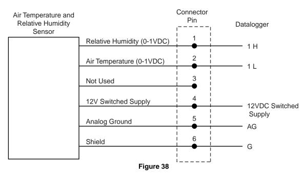
Schematic of RH and Temperature Probe and Connector Temp/RH
