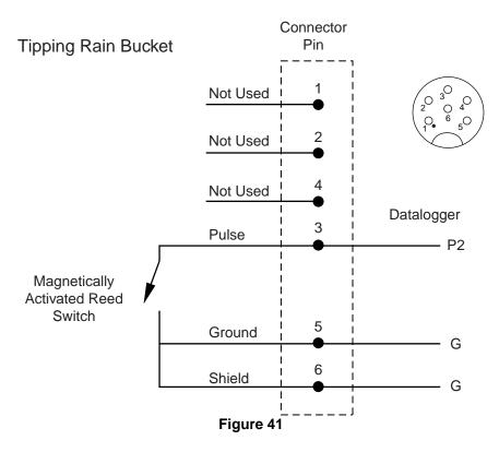
Schematic of Rain Sensor and Connector Rain (Precip)
