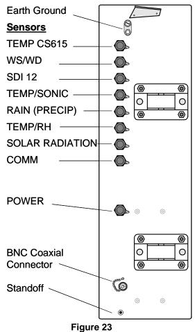
Connect the power and communication cables
