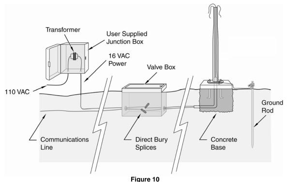
(Note: Figure 10 does not demonstrate the surge protection and grounding requirements for the system)
