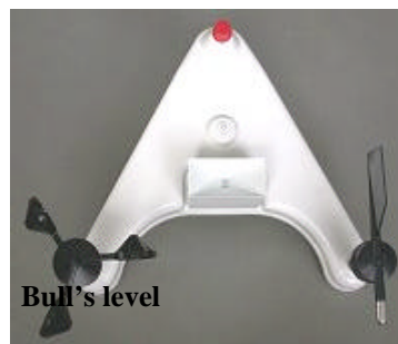
Figure 9 Bull's Level on top of the weather station
